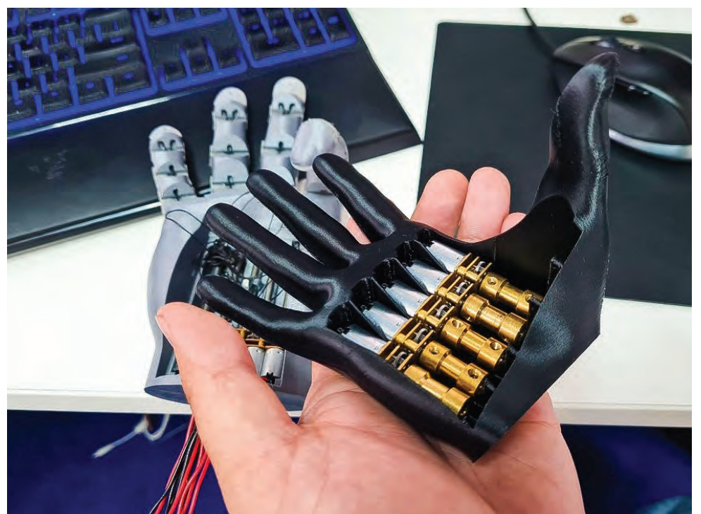
Free 3D Hands is now trying to design a bionic hand and arm from readily available components, to make them affordable for children. The challenge is fitting the existing components into the small hand.
