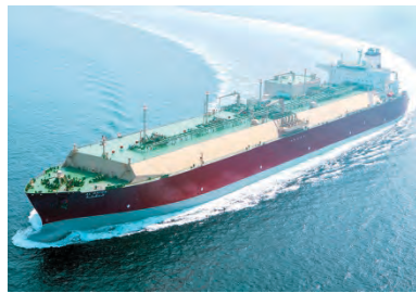
An example of a floating storage and regasification unit and liquid natural gas ship. AGL's plans would see liquified natural gas transported on up to 40 LNG super tankers – about 300 metres long, 49 metres wide – per year from interstate and overseas. Image: Höegh LNG.
