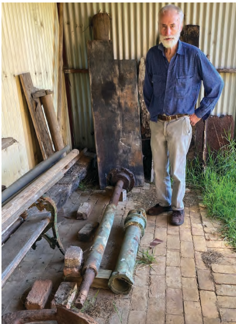
The 3 inch diameter iron propellor shaft and bronze stern tube from the ferry Ventnor is now owned by the Phillip Island Historical Society, but are being safely stored by Society member and island maritime expert John Jansson (pictured). The stern tube went through the timber stern post and carried the propellor shaft, acting as a bearing for the shaft and a seal to prevent leakage of water.
