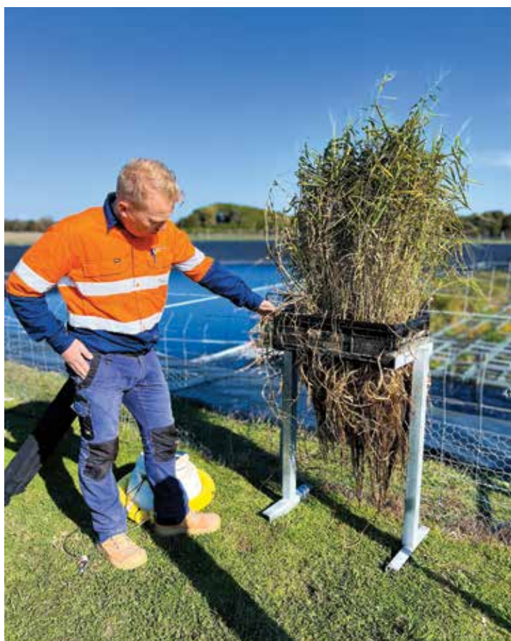
Left: Mark Dishon, Westernport Water next to a tray of Common Reed which accumulated the highest amount of emerging contaminants. Top Right: A cross section diagram of a constructed floating wetland system. Bottom Right: Pictured from left Divina Navarro, CSIRO; Dr Christopher Walker, Covey Associates Pty. Ltd.; Dr John Awad CSIRO; Meg Humphrys, Water Services Association of Australia; Zoe Geyer, Westernport Water; Peter Macreadie, Deakin University Blue Carbon Lab and Dr Lukas Schuster, Deakin University's Blue Carbon Lab.
