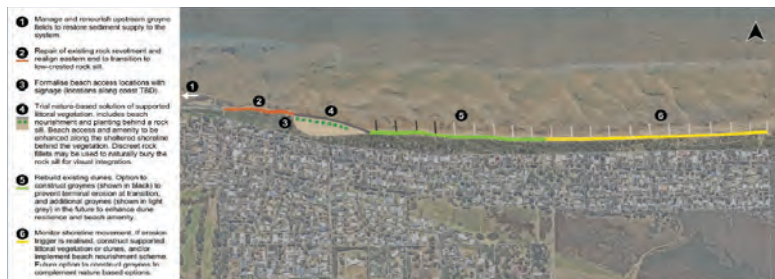
This map, on page 39 of the final East Cowes and Silverleaves Adaptation Plan, shows the planned actions to protect Silverleaves from erosion, including an artificial rock sill (4) and potentially groynes in the future (5).
